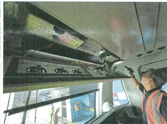
20 August 2024 : G4 Trainset 4 Driver's Cab Water leak Test at Baclaran Depot
