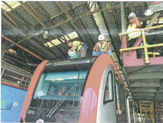
20 August 2024 : G4 Trainset 4 Driver's Cab Water leak Test at Baclaran Depot
